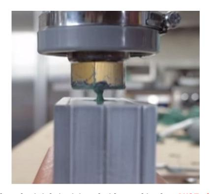
Here molten plastic is being injected with a machine from **LNS Technologies**
