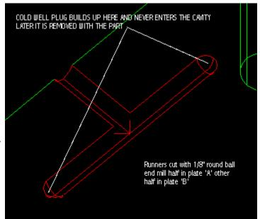
carry the melted plastic from the machine to the pocket, but they don't just dump it into the cavity, rather they stop just past it. Yes, that is right, the runners carry the molten plastic right past our cavity. The runner dead ends in and area called a *cold well*. As molten plastic travels into our mold and down the runners under substantial pressure, area in contact with the walls of the runner begin to cool slightly and the
