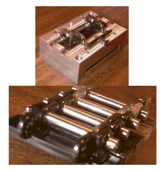
Many of the SRS members have the abilities and machinery necessary to make minimal injection molds. The next time the need arises for numerous plastic parts weather spacers, washers, Lego blocks, or tractor treads I hope you will consider this as a viable option to choose from your toolbox.
