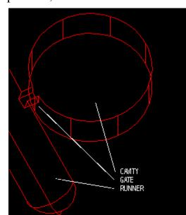
leading plastic builds up a plug of cooled plastic. The plug more properly called a *cold plug* flows right past the small entrance to our mold cavity, and gets trapped in the cold well.
