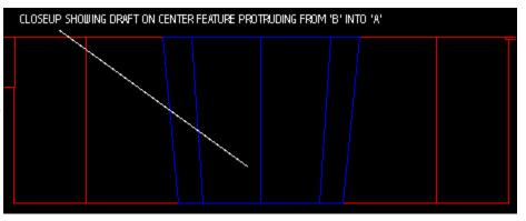
with a bit of an angle. (fig. 10, note that the piece sticking down into the part to form the center hole {blue} of this 'washer' actually sticks out of the other half of the
