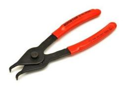
The barrel assembly is held in place in the Model 150A by an external snap-ring. The easiest way to remove and install the snap-ring is to use Angled External Snap-Ring Pliers
